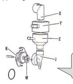
Every day, at the end of the day, disassemble the parts that compose the mixer unit ('X', 'Y', 'Z', 'K', 'J' and the internal plastic impeller 'W') and therefore wash them with hot water.
